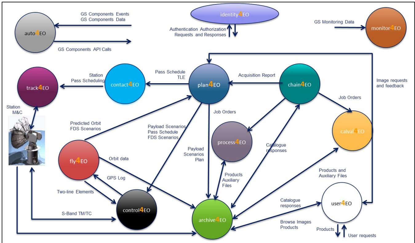
The figure above outlines the most typical GS set-up using all **gs4EO** elements, providing full ground segment capabilities required by any EO mission. With this solution, customers would mainly access the S/C resources via the User Services, and all tasking, data downlink and processing would be performed autonomously by the remaining elements, ensuring complete user feedback throughout every step.
